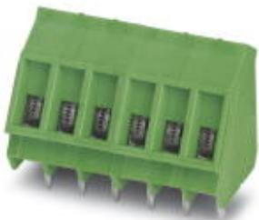
PCB terminal block, nominal current: 24 A, pitch: 5 mm, number of positions: 6, connection method: Screw connection with tension sleeve, mounting: Wave soldering, conductor/PCB connection direction: 55 °, color: green. The article can be aligned to create different nos. of positions!
